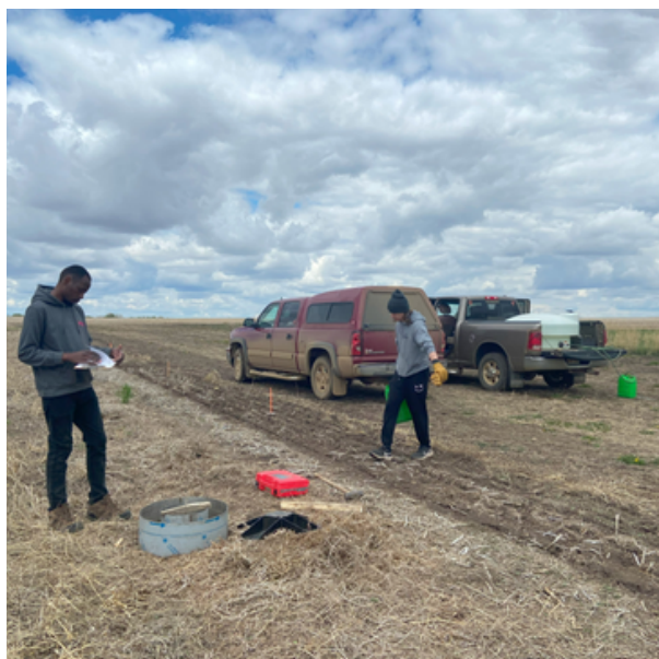
THE DOUBLE RING INFILTROMETER IN CANOLA STUBBLE. MULTIPLE INFILTRATIONS REQUIRE LARGE QUANTITIES OF WATER. PHOTO BY ALEXANDER OLSON
