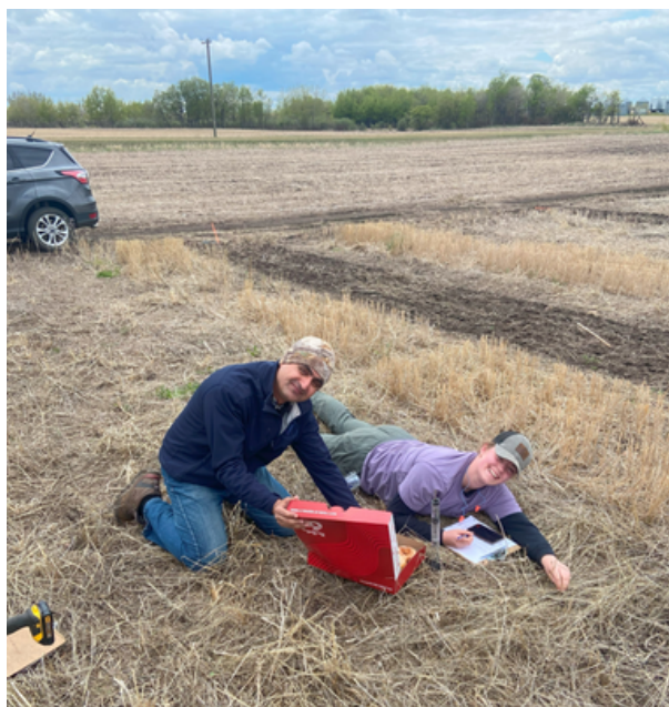
THE MINI DISC INFILTRMETER IS A SMALL TUBE THAT TESTS THE INFILTRATION RATE ON SMALL AMOUNT OF SOIL. PHOTO BY ALEXANDER OLSON
